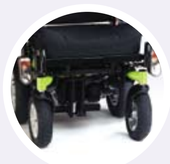
Single arm front fork with improved design to limit damage from impacts
